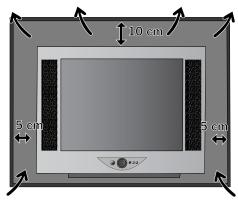
If the TV set is placed in a cabinet or on a shelf, at least 5 cm clearance at the sides and at least 10 cm at the top must be left to allow air to circulate.
